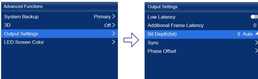
Step 2 Select **Bit Depth** and then select the desired bit depth value from the drop-down options.
