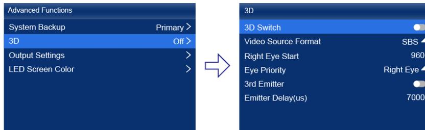
Step 2 Turn on the 3D function by setting the 3D switch to
