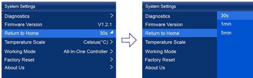
Step 2 Select **30s**, **1min** or **5min** from the drop-down options as required.
