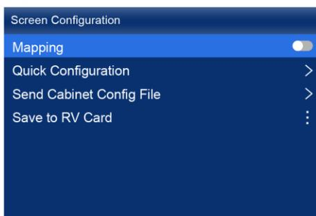
Step 2 Enable the Mapping function by toggling on this switch
